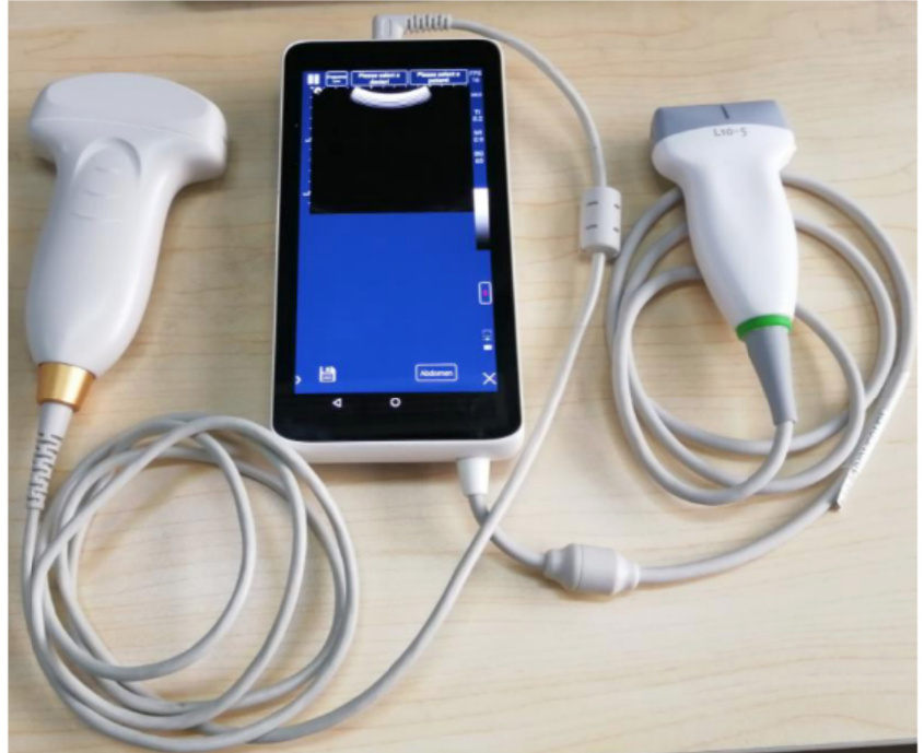
VMX-MU3LC Plus supports 2 probes: 1 fixed Linear probe, and 1 USB Convex probe
